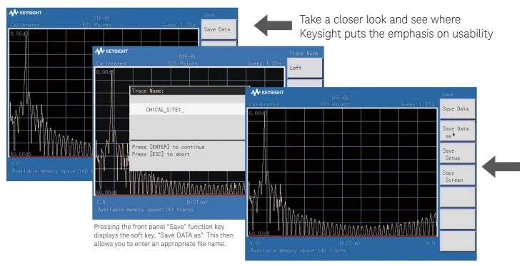
Subsequently, press the "Save DATA" soft key, each new file name automatically increments, as in example: CHICAG\_SITE2, CHICAG\_SITE3,...
