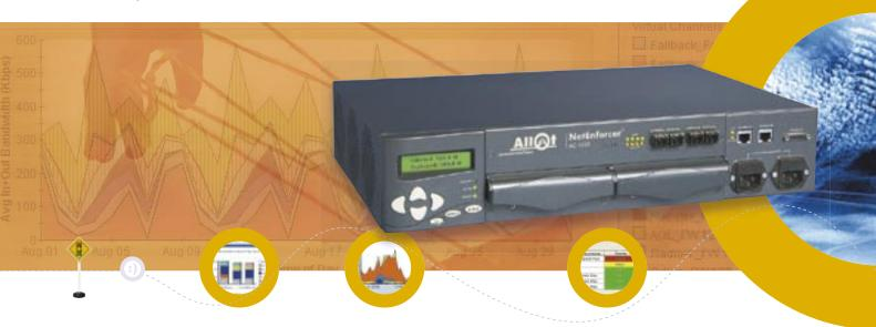
Allot NetEnforcer AC-1000 series is especially suitable for managing Internet traffic on high-speed Ethernet links of up to 2 Gbps. Using deep packet inspection (DPI) technology with policy based QoS enforcement, they monitor and control network usage, optimize service delivery, and provide an unsurpassed level of visibility.
