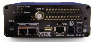
Cricket QAM Plus offers an 1 GHz RF interface with a Dual Tuner, 10/100Mb Ethernet ports and plug & play USB for connection to any PC.
