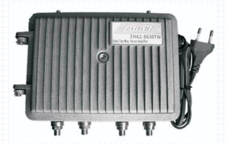
The single-output amplifier features variable gain and slope controls, as well as attenuator and equalizer facilities for greater flexibility when adjusting the amplifier. Both input and output ports are standard 5/8-24 entry ports for added flexibility. The ZHA2-8630TW ships standard with built-in diplex filters at its input and output. It includes an active return path for use in today's advanced networks.
